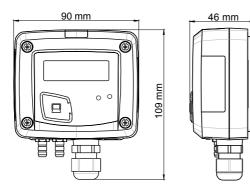
Material : ABS V0 as per UL94 Protection : IP65 Display : LCD 10 digits. Size : 50 x 17 mm Height of digits : Value : 10 mm ; Unit : 5 mm Connections : ribbed, Ø 6.2 mm Cable gland : for cables Ø 8 mm maximum Weight : 143 g
