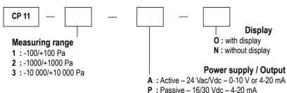
Example : CP 113 – AO Pressure transmitter measuring range -10 000/+10 000 Pa, 0-10 V or 4-20 mA active, with display
